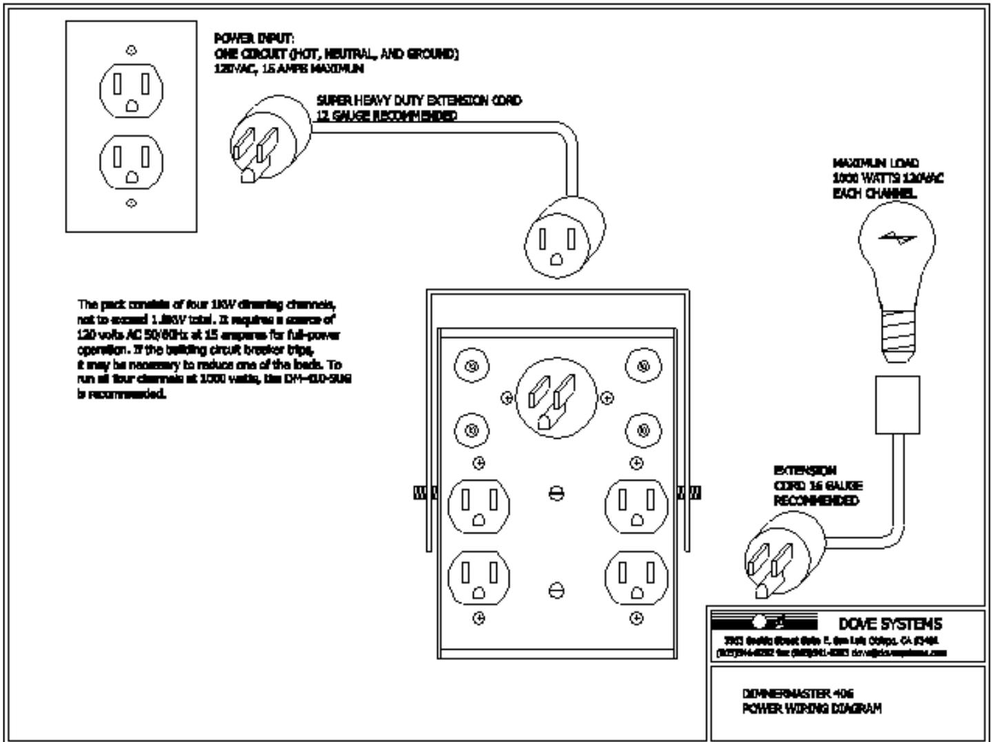
Power input to the pack is via a flush-mount male connector on the back panel. Any standard heavy-gauge extension cord will work for this purpose. Always use 3-wire, grounded cables. 12AWG cable is recommended.
